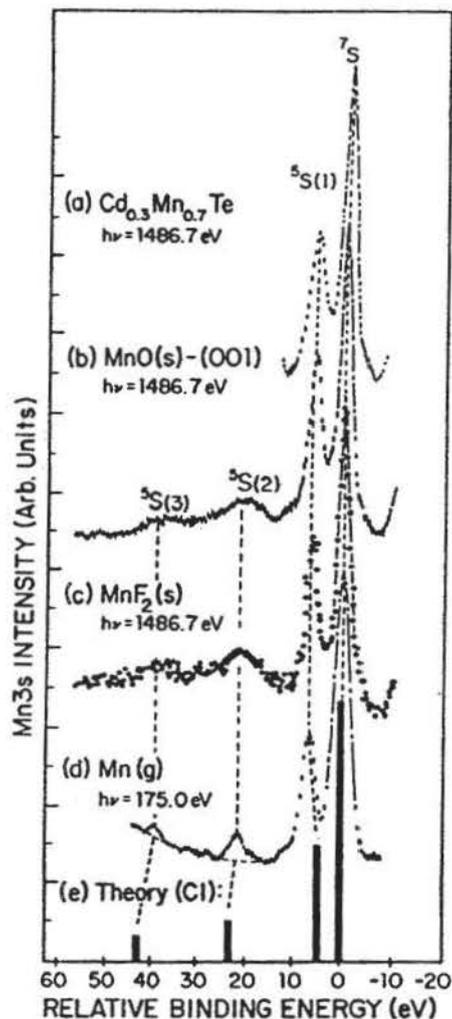
FIGURE 40. Experimental Mn 3s spectra for (a) the diluted magnetic semiconductor  $\text{Cd}_{0.3}\text{Mn}_{0.7}\text{Te}$ , (b) MnO (001), (c) polycrystalline  $\text{MnF}_2$  (Ref. 139), and (d) gaseous atomic Mn are compared to (e) theoretical calculations for emission from a free  $\text{Mn}^{2+}$  ion including final-state configuration interaction (Ref. 140). (From Ref. 138.)
