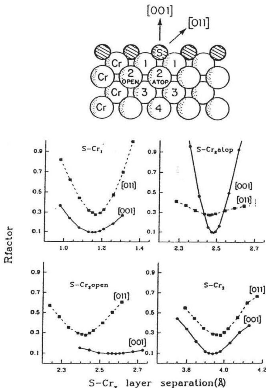
FIGURE 21. *R*-factor analysis of the scanned-energy results of Fig. 20, showing the geometry involved and the variation of the *R* factor with various S-Cr layer separations. (From Ref. 20.)
