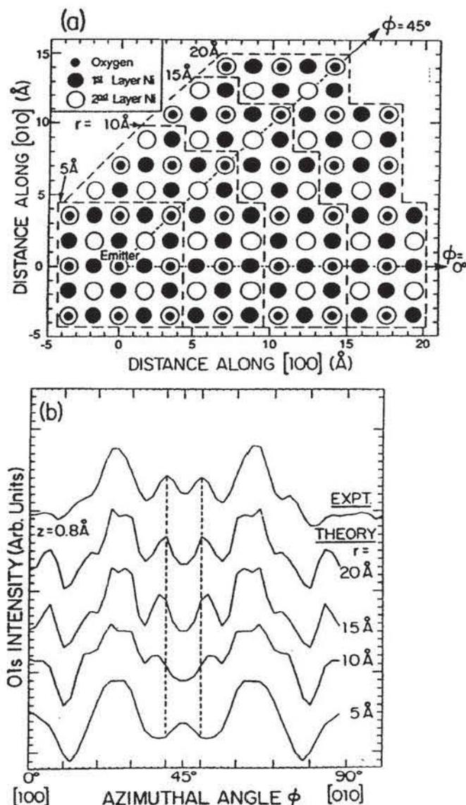
FIGURE 16. (a) Choices of cluster. Different-sized clusters used in testing the convergence of the SSC-SW curves for  $\theta = 8^\circ$  in Fig. 15(a), labelled with the approximate radii outward from the emitter that they represent. (b) Convergence with cluster size. Calculated curves for the clusters of (a) with  $z = 0.8 \text{ \AA}$  are compared to experiment. Note that a radius of at least  $20 \text{ \AA}$  is required to yield optimum agreement. (From Ref. 26.)
