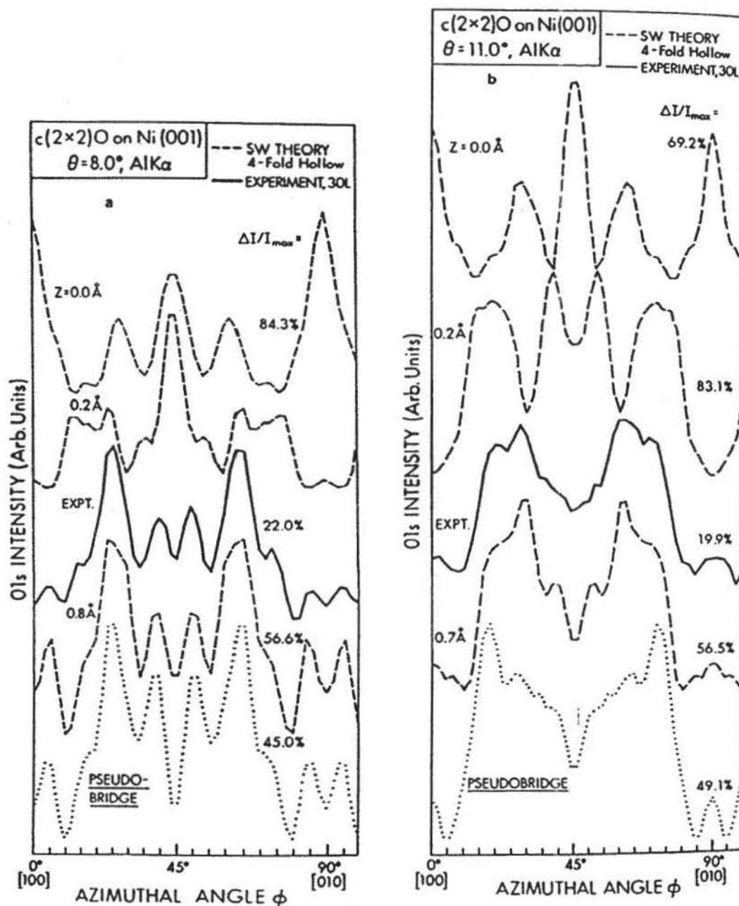
FIGURE 15. (a) Grazing-emission O 1s azimuthal data from  $c(2 \times 2)$  O on Ni (001) at  $\theta = 8^\circ$ . The experimental data are compared to SSC-SW curves for four possible fourfold-hollow  $c(2 \times 2)$  structures, including the pseudobridge geometry of Ref. 98. (b) As in (a), but for  $\theta = 11^\circ$ . (From Ref. 26.)
