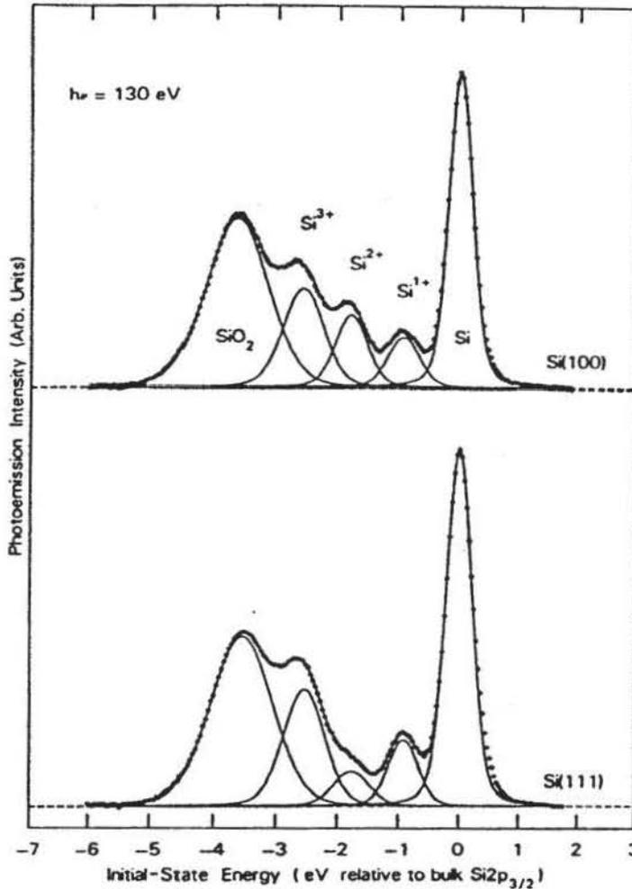
FIGURE 35. The Si  $2p_{3/2}$  components of Si 2p spectra from thin oxide films of approximately 5 Å thickness thermally grown on Si (100) and Si (111) surfaces. Note the reduced intensity of Si<sup>2+</sup> for Si (111), assumed to be due to structural differences in the interface. [From Ref. 123(c).]
