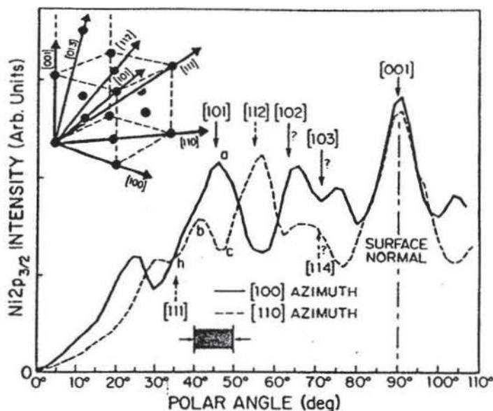
FIGURE 38. High-resolution  $\text{AlK}\alpha$  polar scans of  $\text{Ni } 2p_{3/2}$  intensity above  $\text{Ni } (001)$  in two different azimuths, with certain low-index directions and special points noted [cf. lower-case letter labeling in Fig. 37(c)]. The region covered by Fig. 37(c) is shaded. The inset shows the near-neighbor/low-index directions within an *fcc* unit cell. (From Ref. 48.)
