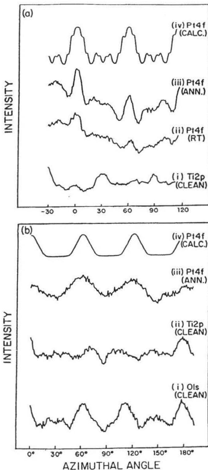
FIGURE 33. (a) Azimuthal XPD data for Pt 4f and Ti 2p emission from Pt on  $\text{TiO}_2$  (110) at  $\theta = 40^\circ$  are compared to PW cluster calculations including double scattering for Pt emission from a (111)-oriented metal cluster of about 15 Å diameter. Al  $K\alpha$  radiation was used for excitation. (b) As in (a) but for Pt 4f, Ti 2p, and O 1s emission from Pt on  $\text{TiO}_2$  (100) at  $\theta = 45^\circ$ . (From Ref. 120.)
