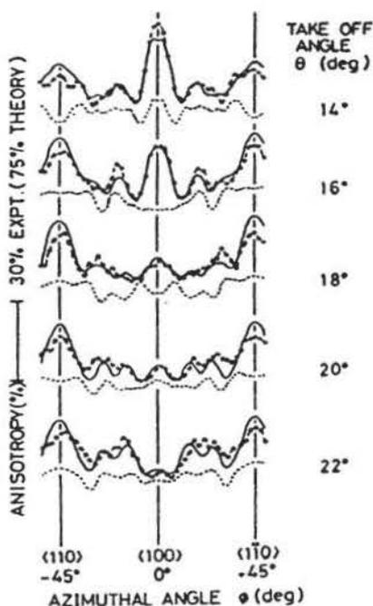
FIGURE 29. Azimuthal data for Al  $K\alpha$ -excited K  $2p$  emission from the Si (001)  $(2 \times 1)$  surface saturated with K at polar angles from  $14^\circ$  to  $22^\circ$  above the surface. Experiment is compared with SSC-PW calculations for the two models shown in Fig. 28: ODAC = dashed curves and DL model best fitting data = solid curves. Very similar curves were also obtained with SSC-SW calculations. (From Ref. 114.)
