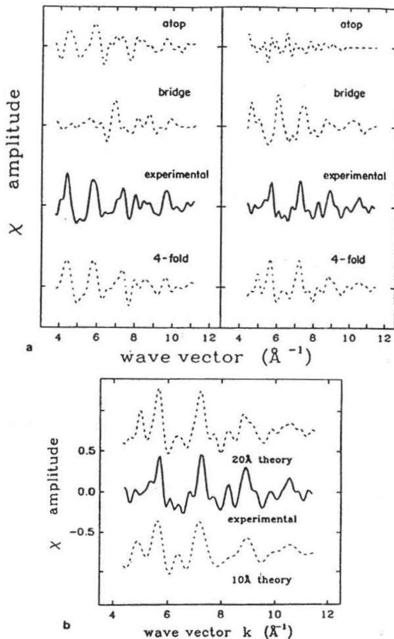
FIGURE 20. (a) Comparison of scanned-energy S 1s experimental data for emission from  $c(2 \times 2)$  S on Cr (001) along the [001] direction (left panel) and [110] direction (right panel) with MSC-SW calculations for different adsorption sites of atop, bridge, and fourfold. (b) As in (a), but comparing the data obtained in the [011] azimuth to MSC-SW theory for the final optimized fourfold-hollow structure with different path-length cutoffs of 20 Å and 10 Å. (From Ref. 20.)
