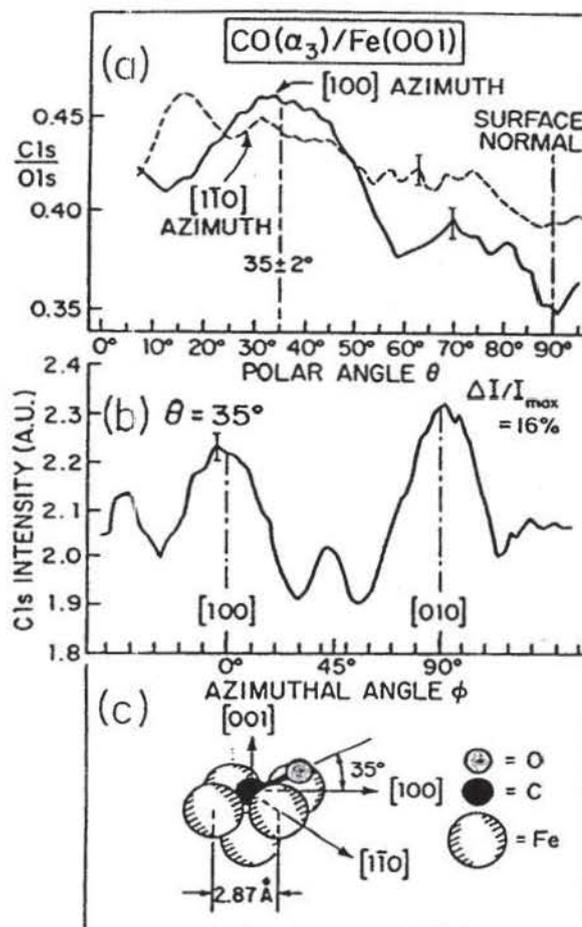
FIGURE 9. (a) Experimental polar scans of the C 1s/O 1s intensity ratio for the  $\alpha_3$  state of CO on Fe (100). The C 1s kinetic energy is 1202 eV. Curves are shown for two azimuths: [100] (solid curve) and [1,  $\bar{1}$ , 0] (dashed curve). (b) Experimental azimuthal scan of C 1s intensity for the  $\alpha_3$  state of CO at a polar angle of  $35^\circ$  chosen to coincide with the peak in the [100] data of part (a). (c) The bonding geometry as deduced from these data. (From Ref. 86.)
