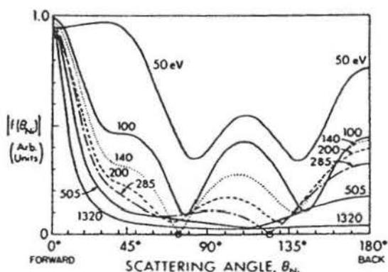
FIGURE 2. Nickel plane-wave scattering factor amplitudes  $|f_{Ni}|$  as a function of both the scattering angle  $\theta_{Ni}$  and the photoelectron kinetic energy. Note the zeroes occurring for both 140 eV and 285 eV, which have been termed a generalized Ramsauer-Townsend effect. (From Ref. 21.)
