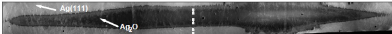
MEM 28 μm x 350 μm; after 130 L NO<sub>2</sub>;
