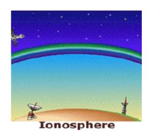
Upper ionized region of the atmosphere known as Ionosphere (from 60–800km approx.) acts as a mirror for High Frequency Radio Waves (3-30 MHz) so that Long Range Communication becomes possible.
