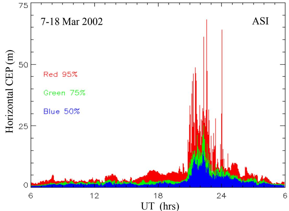
Single point positioning error (2D) better than 10 meters 95% of the time ... except during scintillation
