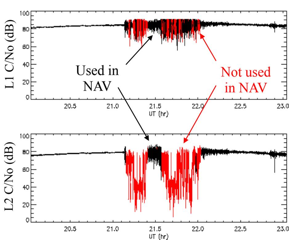
Scintillation Causes Fading of L1 and L2 GPS Signals
