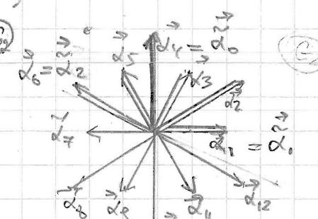
$$\begin{aligned} \vec{\alpha}_4 &> \vec{\alpha}_3 \Leftrightarrow \vec{\alpha}_4 - \vec{\alpha}_3 = \vec{\alpha}_5 \\ \vec{\alpha}_4 &> \vec{\alpha}_2 \Leftrightarrow \vec{\alpha}_4 - \vec{\alpha}_2 = \vec{\alpha}_6 \\ \vec{\alpha}_4 &> \vec{\alpha}_1 \Leftrightarrow \vec{\alpha}_4 - \vec{\alpha}_1 = \vec{\alpha}_6 + \vec{\alpha}_3 \\ \dots \end{aligned}$$
