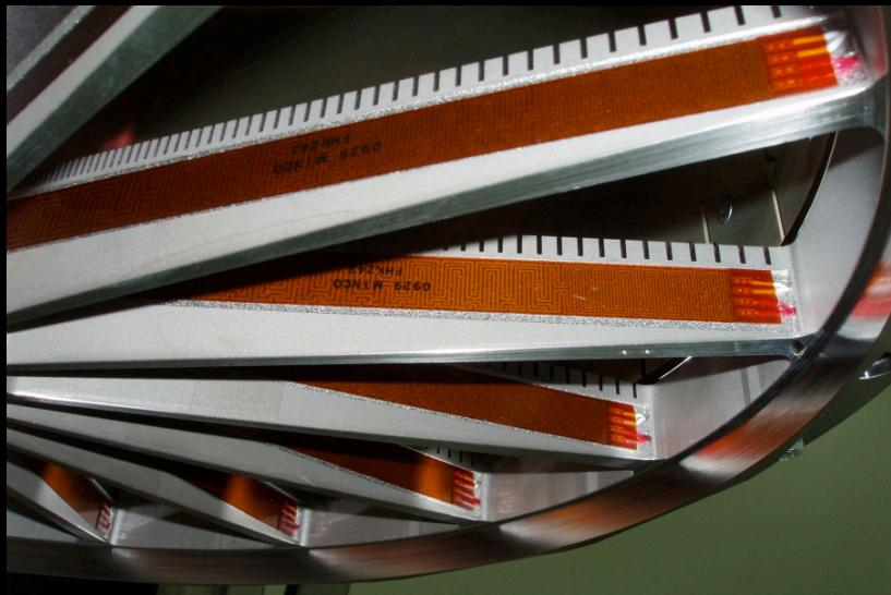
Spider Wheel with heaters integrated
