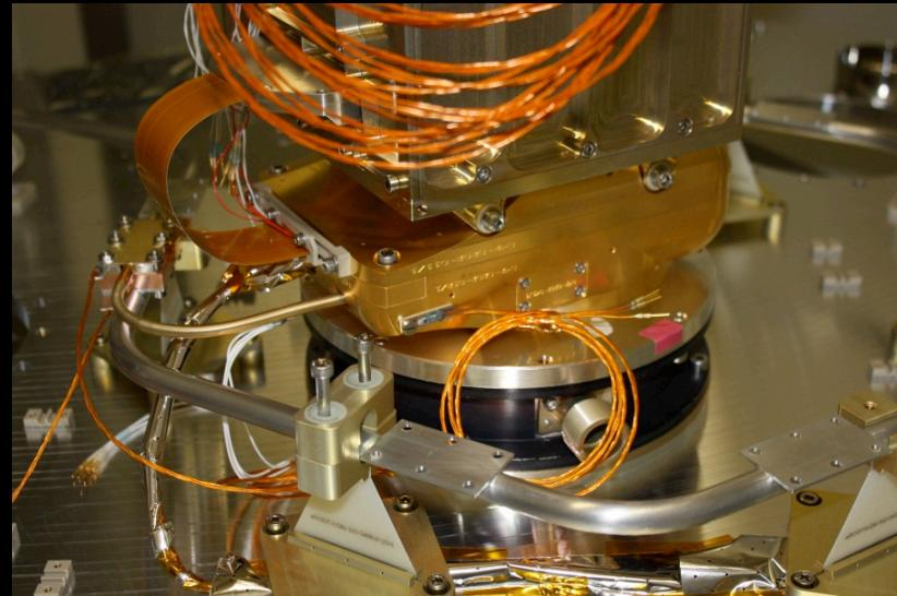
Preparation of Thermal Test with Heatpipe System
