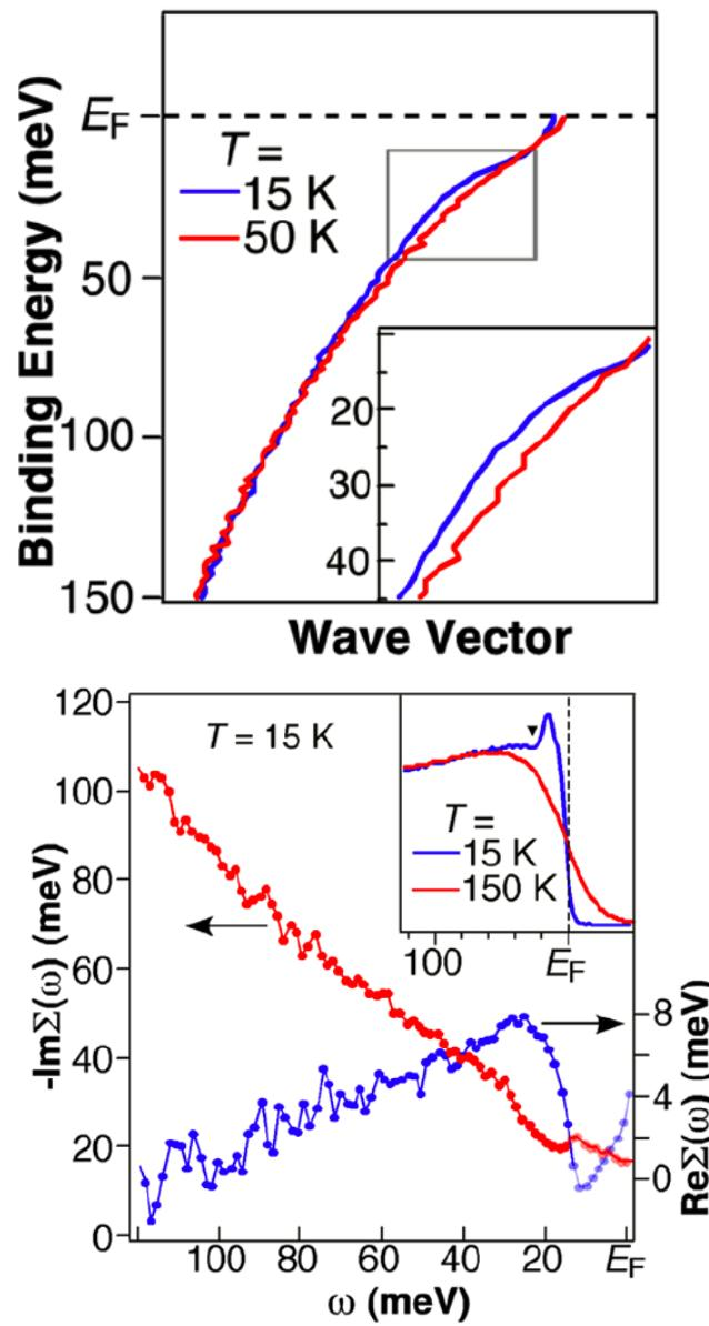
$\Omega \sim 13 \text{ meV}$ , similar to neutron resonance mode  $\sim 14 \text{ meV}$
