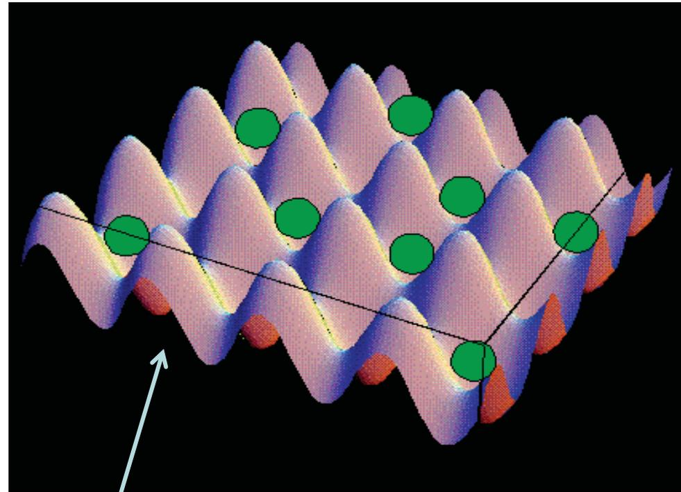
Electric fields in a laser induce a dipole moment which interacts with the field: schematic of a potential felt by the atoms
