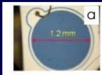
Hamamatsu S5821 p-i-n diode
