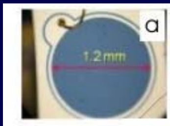
Hamamatsu S5821 p-i-n diode
