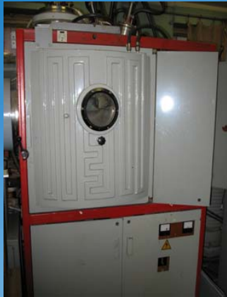
Equipment for deposition (VU-2MBS)
