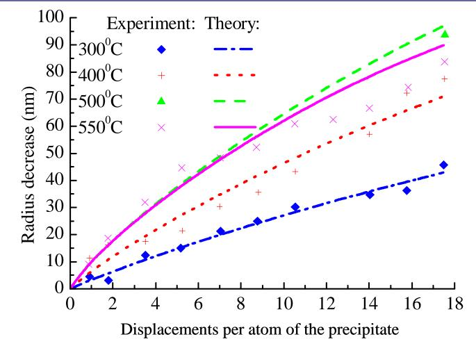
Decrease of the radius of MgO-based precipitates under 1 MeV electron irradiation [I. Monnet et al. JNM (2004) **335**, 311]
