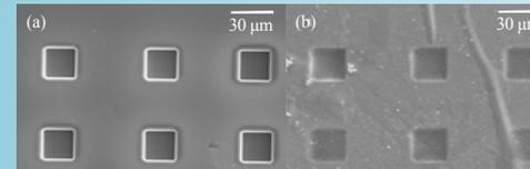
SEM is extensively used to detect the trenches which are now covered by the SSF. A SEM picture shows the image (top view) of (a) trenches fabricated on a Si silicon, (b) the trenches covered by the SSF.
