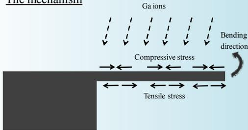
Defects, vacancies are formed at the surface of the cantilever by the ions. The unstable/perturbed atoms at the top layers try to reconfigure themselves, generating different amounts of stress in different layers of the system. The reconfiguration process initiates the bending of the structure.
