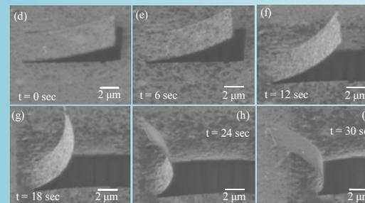
Ion beam is irradiated on the cantilever. The cantilever tends to bend towards the ion beam side.
