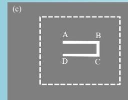
Schematic picture shows the fabrication procedure of a cantilever. The cantilever is fabricated at the mid of the SSF by milling out the portion along the AB, BC and CD line (figure c). The dotted line indicates the location of the trench.
