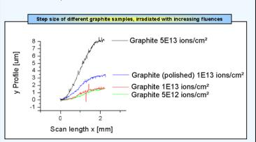
Investigation of irradiated isotropic graphite samples shows a radiation induced swelling of the sample. Analysis of the experiment shows that below a critical fluence of around 2×10  $^{\rm 13}$  ions cm $^2$  the swelling effects are small.
