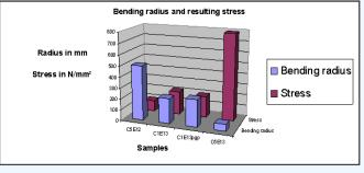
Swelling induced stresses were calculated with the obtained data from the DEKTAK profilomete
