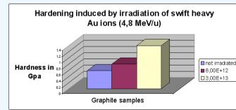
The material hardens under the swift heavy ion irradiation due to the aggregation of structural defects and grain and domain boundaries which are obstacles for dislocation[3]. Hardening also points to the formation of other carbon structures like glassy carbon inside the swift heavy ion irradiated graphite[3].
