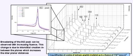
Investigation of irradiated using a synchrotron X-ray source, show the influence of radiation damage on the structure.
