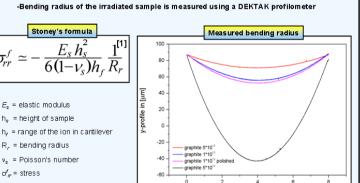
Analysis of irradiated isotropic graphite cantilevers with a profilometer show the results of the radiation induced stress in the form of a bending of the samples. Above a critical threshold of a fluence about  $2\times10^{13}$  ions cm  $^2$  the swelling induced stress is significantly increased. This is indicated by the increase of the bending radius.
