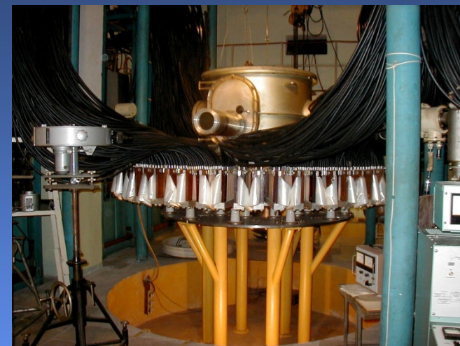
Capacitive storage (left) & chamber with current collector (right)
