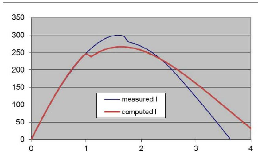
Figure 2.4 Fitting of computed current to measured current waveform by adjusting  $L_0$
