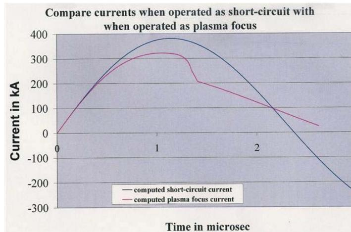
**Figure 1.3** Plasma focus current is distorted from unloaded current wave form.
