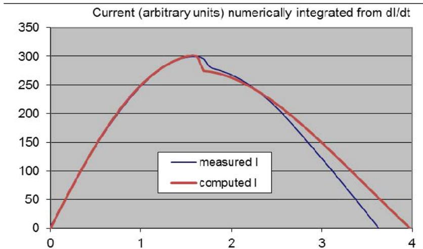
**Figure 2.5** Improved fitting of computed current to measured current by adjusting for effective ‘straight length’ channel  $z_0$
