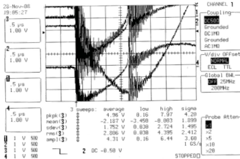
Fig. 89 Oscilloscope traces of the discharge current derivatives in a property-sheet mode of the DPF operation obtained at all 4 PSSs
