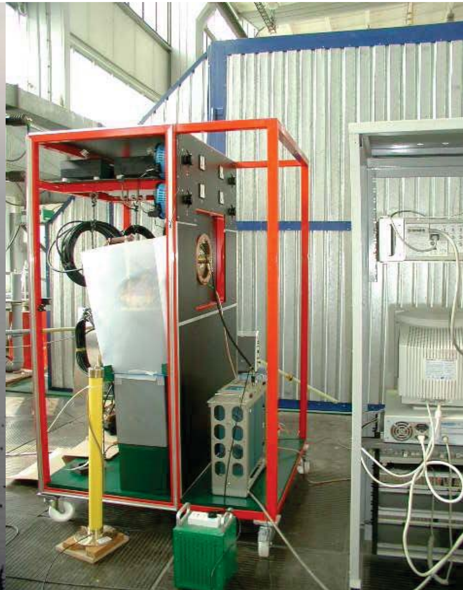
Transportable device PF-6: 7 kJ, 750 kA, 10^9 D-D or 10^{11} D-T n/pulse, weight – 400 kg (IPPLM + MPS)
