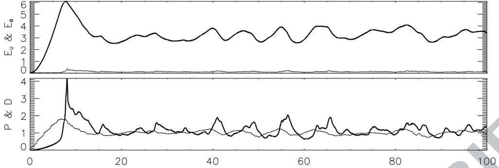
Figure 5: Energy and dissipation rate time series. **Upper panel:** Kinetic energy (thin), and total energy (thick). **Lower panel:** Energy dissipation rate (thick) and Poynting flux (thin).
