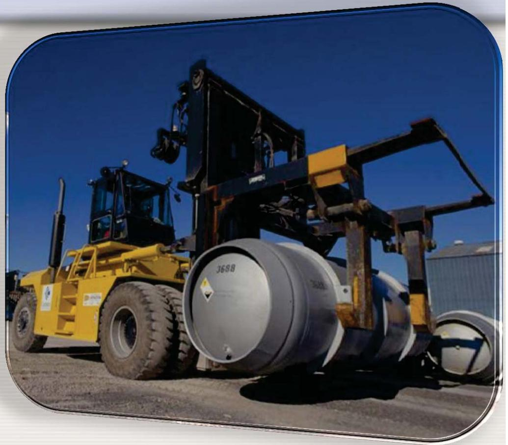
A “48Y” Cylinder containing natural  $\text{UF}_6$
