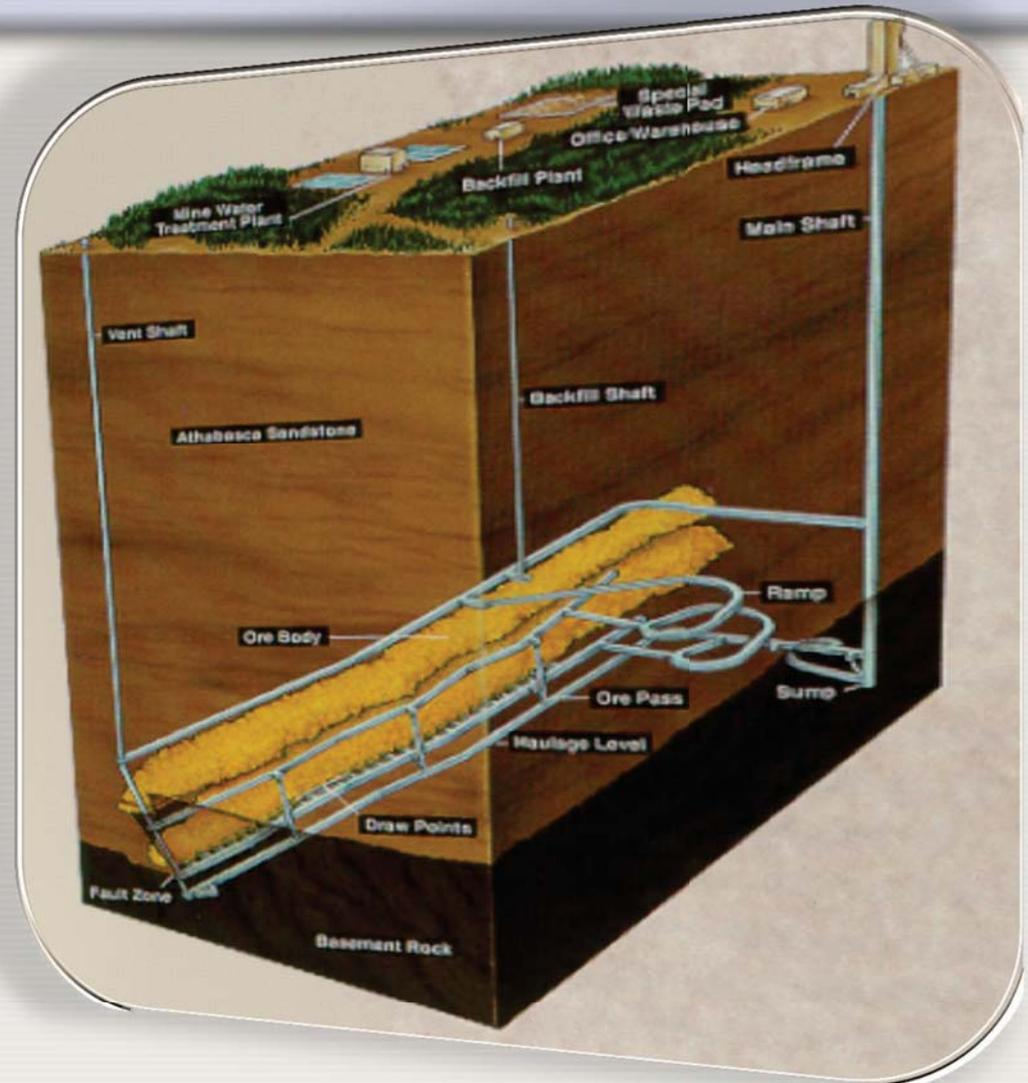
Underground Uranium Mine Schematic
