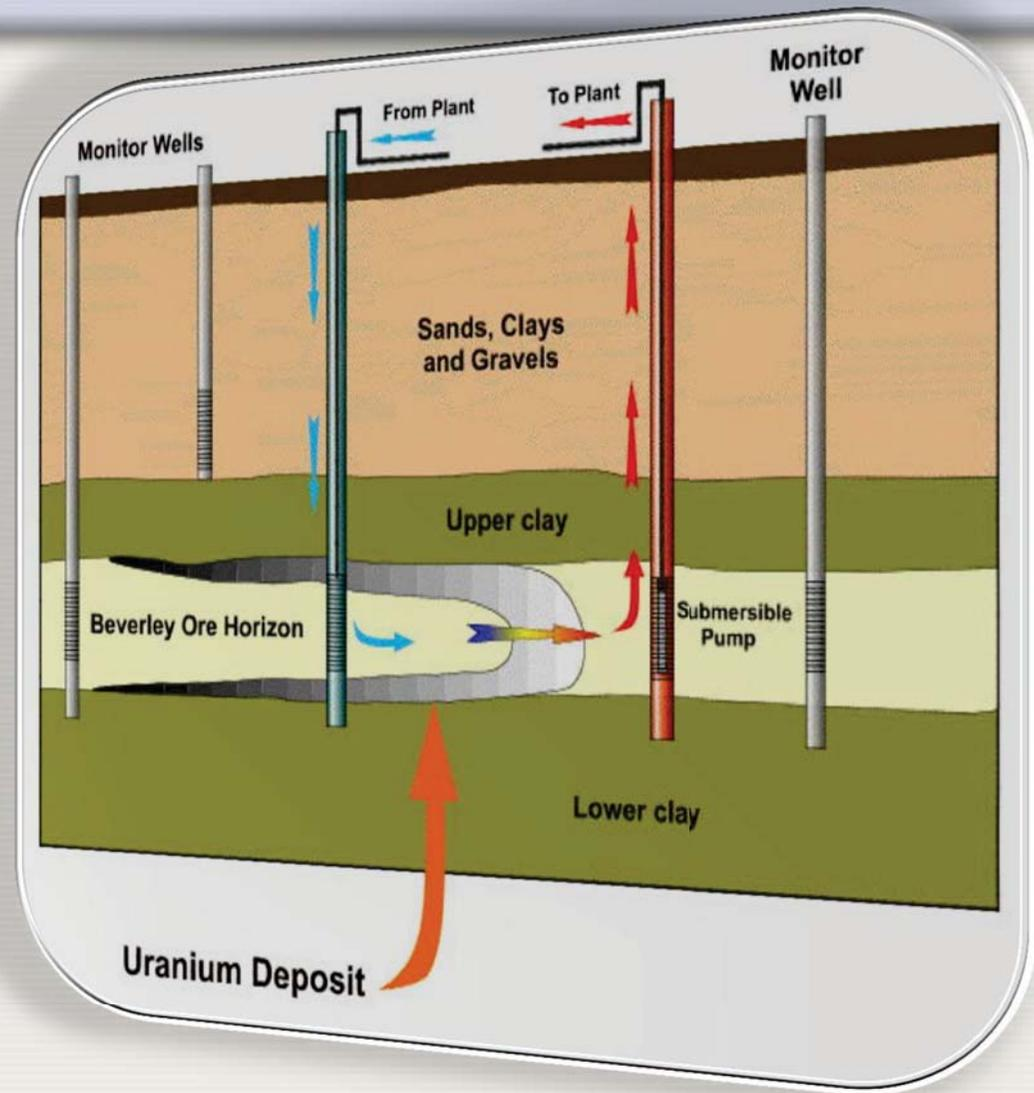
ISL Uranium Mine Schematic
