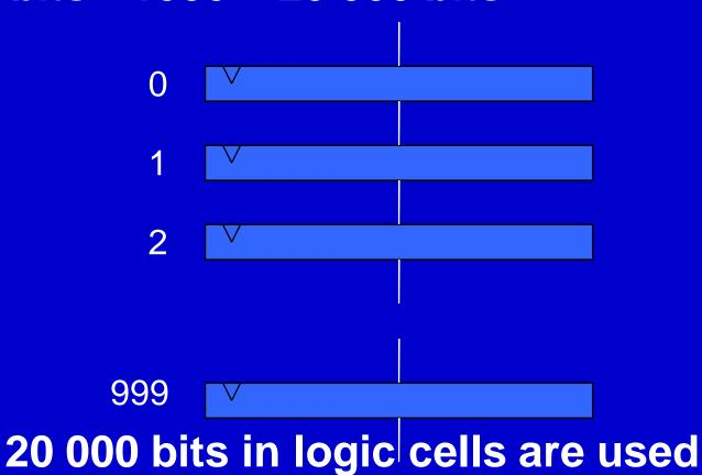
Data pipeline with FIFO based on dual port RAM @ 10 MHz
