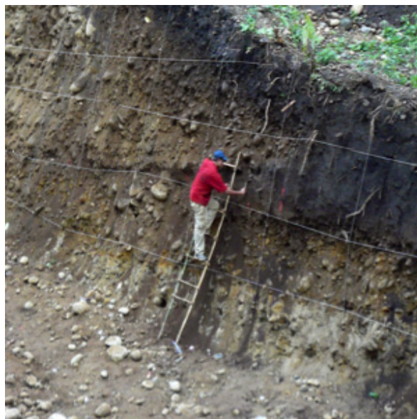
Steve Wesnousky inspecting the Himalayan 1505 earthquake rupture plane (21 m slip M_w \approx 8.9 )
