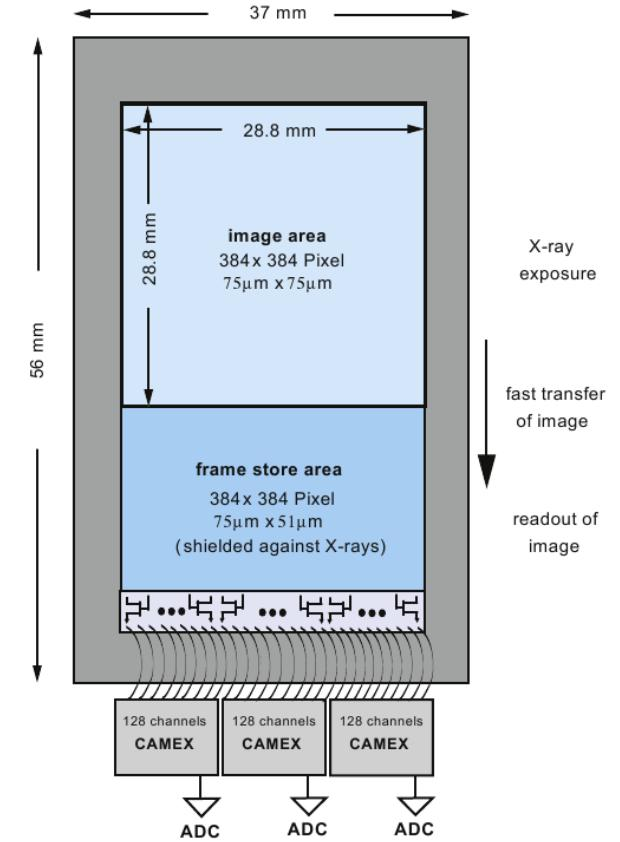
X-ray CCD with 384 x 384 pixels (FoV 1.03 deg)
