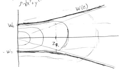
$$\Phi(x,y,z) = kz - \xi(z) + \frac{z}{2z_R} \frac{(x^2 + y^2)}{w^2(z)}$$
