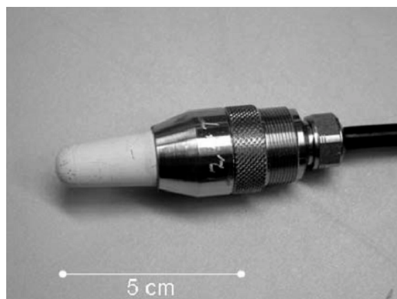
Figure 1. Polymer tensiometer. Source: Durigon; de Jong Van Lier (2011).
