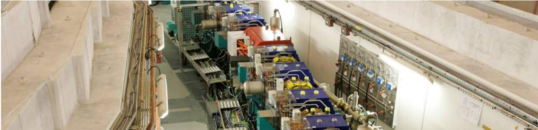
Movable absorbers in the front-end enable each beamline to stop the Xray beam inside the SR tunnel.
