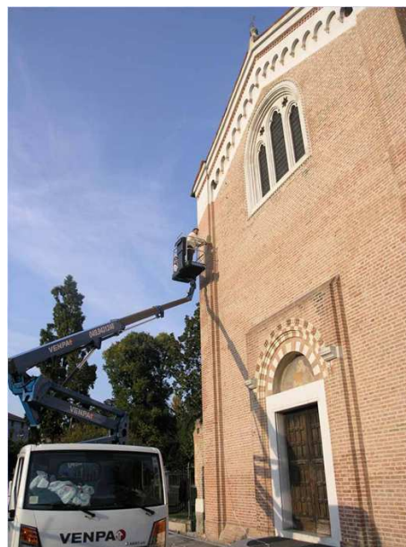
Figure 6: EDXRF sulfur analyses on the Scrovegni facade
