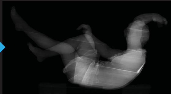
Corrected radiograph (open beam and dark correction)
