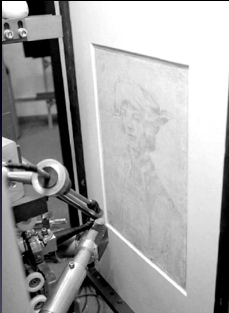
Micro-PIXE measurements of Portrait of Lucas de Leyde by Alfred Dürer A.Duval et al., (Louvre laboratory)
