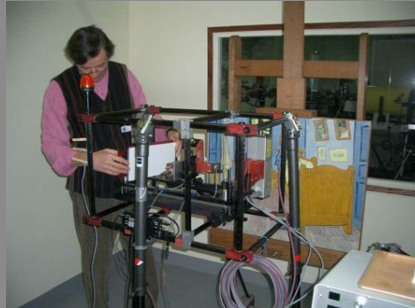
XRD-XRF apparatus in front of a Van Gogh's painting at the C2RMF laboratory
