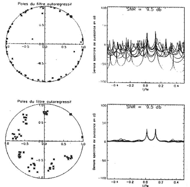
Figure 11. (up) Non-regularized & (bottom) Regularized Doppler AR Spectrum
