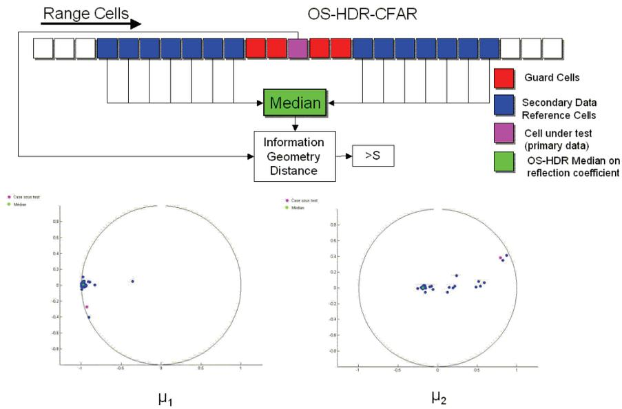
**Fig. 13.** OS-HDR-CFAR Algorithm with illustration of two first reflection coefficients
