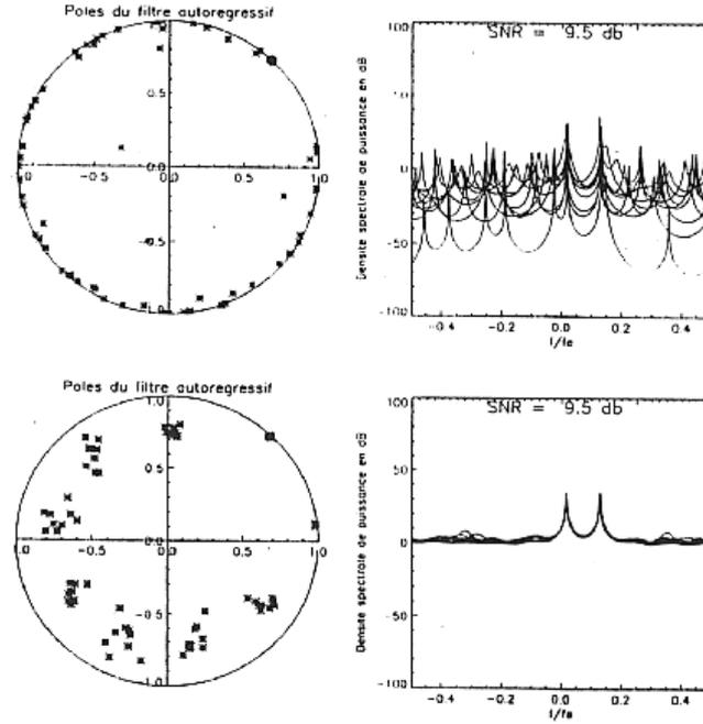
**Fig. 11.** (up) Non-regularized & (bottom) Regularized Doppler AR Spectrum
