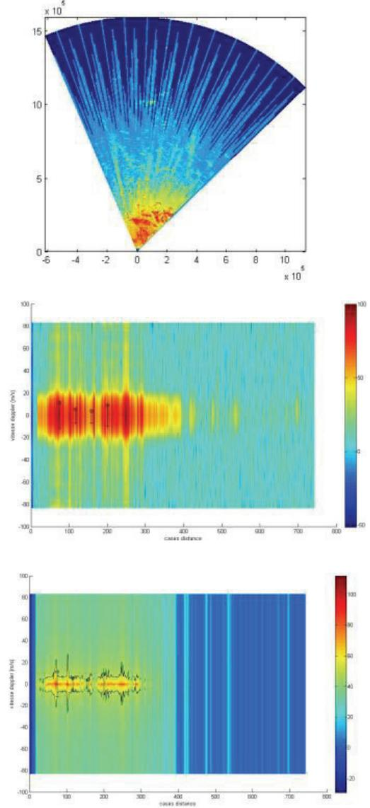
Figure 14. Reflectivity of ground clutter in recorded sector (top), Comparison of FFT Doppler spectrum (middle) and High Resolution Regularized Doppler spectrum (down)
