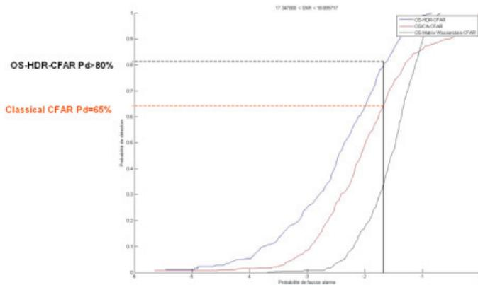
Figure 15. ROC curves for 3 approaches : OS-HDR-CFAR, OS-CFAR/Doppler-Filters, & method based on Wasserstein barycenter/distance (optimal transport theory)
