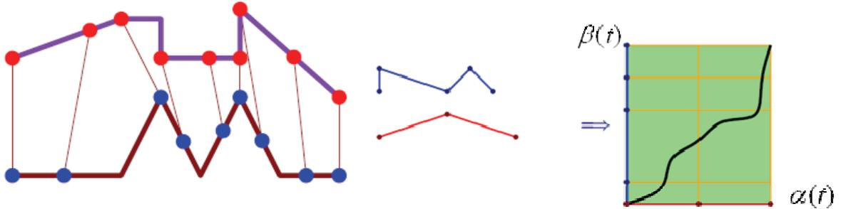
Figure 6. Fréchet Distance between two polygonal curves ( $\alpha$  and  $\beta$  indexing all matching of points)
