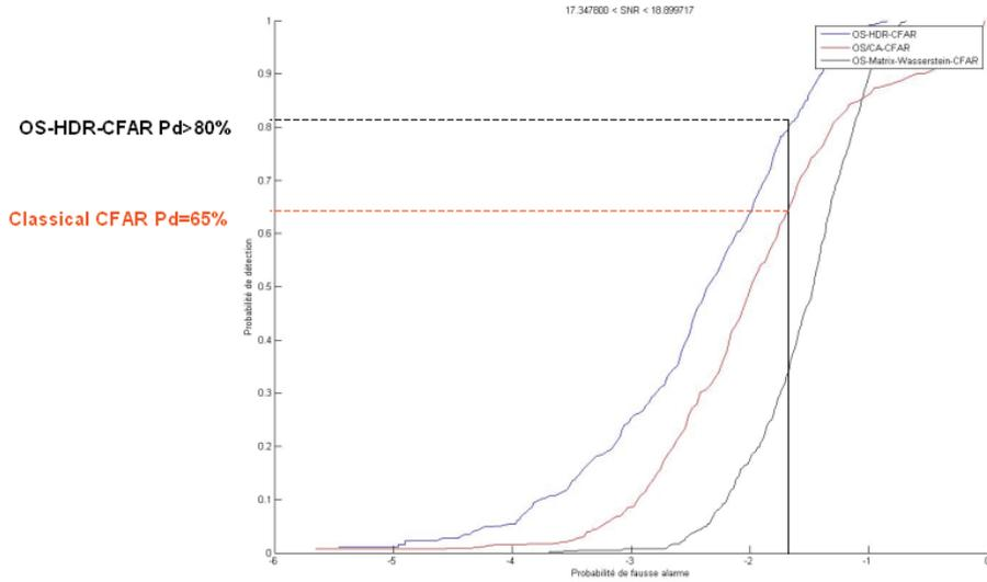
**Fig. 15.** ROC curves for 3 approaches : OS-HDR-CFAR, OS-CFAR/Doppler-Filters, & method based on Wasserstein barycenter/distance (optimal transport theory)
