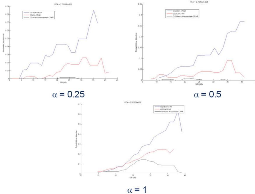
**Fig. 16.** Probability of detection versus SNR for fixed  $P_{fa}=10^{-5}$ , with  $\alpha$  relative position in Doppler of the target normalized by Doppler Clutter Spectrum Width ( $\alpha=1$  means that the target is positioned on the edge in Doppler of the ground clutter)
