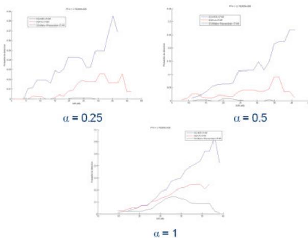
Figure 16. Probability of detection versus SNR for fixed  $P_{fa}=10^{-5}$ , with  $\alpha$  relative position in Doppler of the target normalized by Doppler Clutter Spectrum Width ( $\alpha=1$  means that the target is positioned on the edge in Doppler of the ground clutter)
