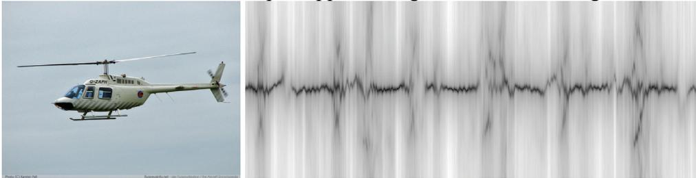
Figure 1. BELL 206 helicopter Time-Doppler Signature in one radar cell in staring mode
