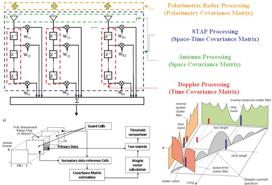
Fig. 10. Doppler Processing, Antenna Processing, Space-Time Processing & Polar processing
