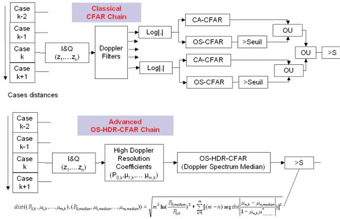
Figure 12. (top figure) Classical OS-CFAR after filter banks, (bottom figure) OS-HDR-CFAR
