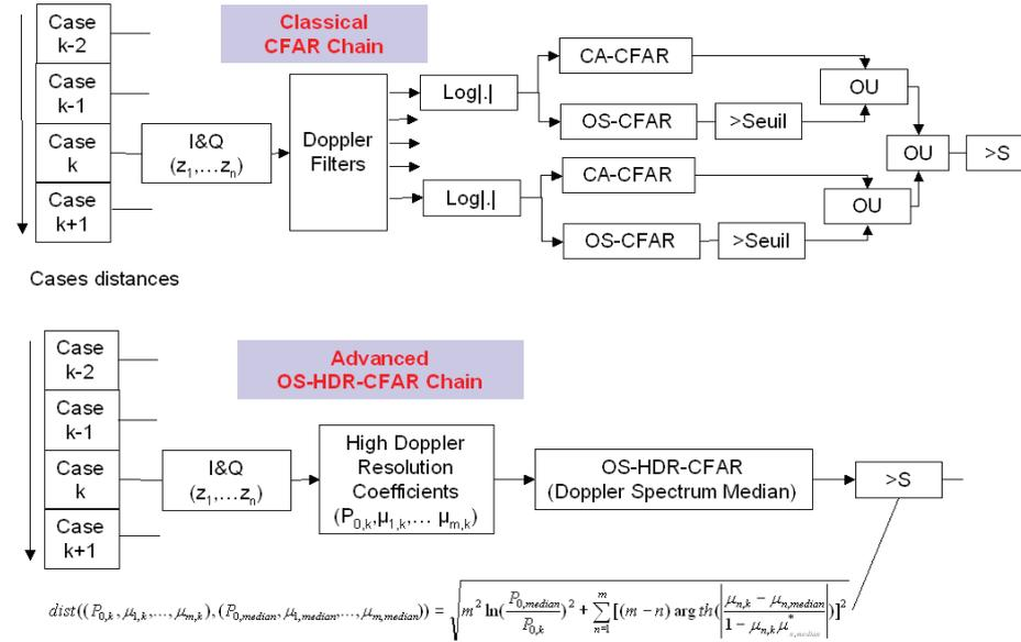
**Fig. 12.** (top figure) Classical OS-CFAR after filter banks, (bottom figure) OS-HDR-CFAR
