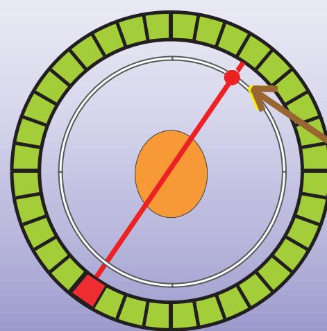
Rotating line source with positron emitter Ge68
