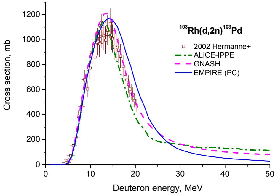
Fig. 9. Experimental data for the  $^{103}\text{Rh}(d, 2n)^{103}\text{Pd}$  reaction cross-section in comparison with calculations by different codes.
