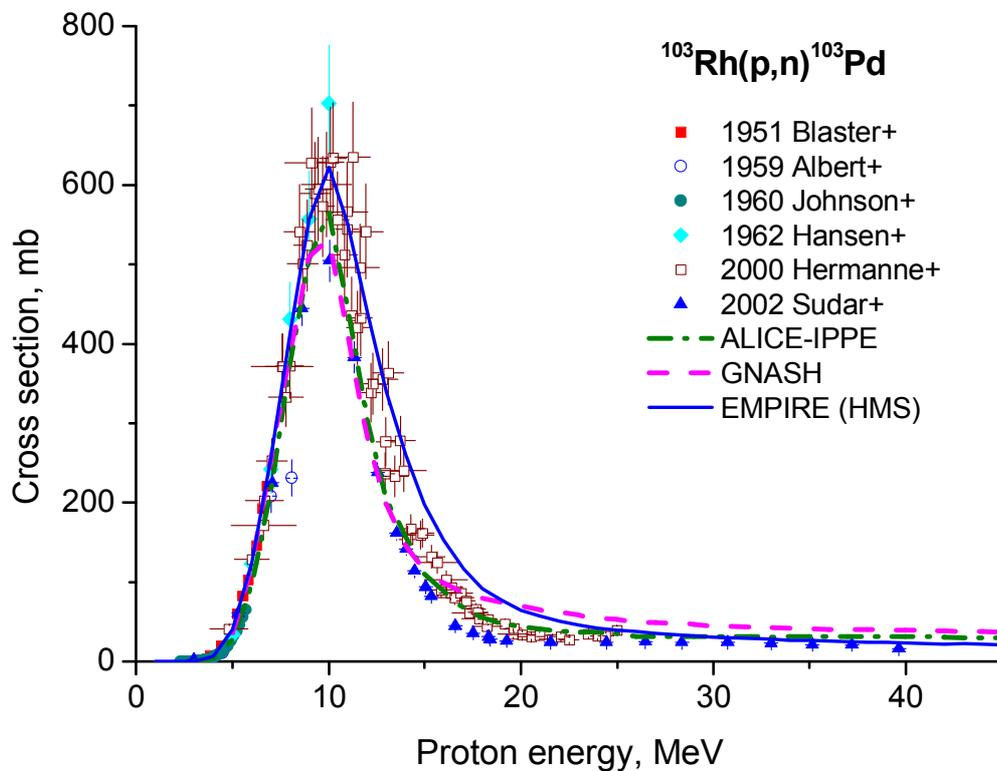
Fig. 8. Experimental data for the  $^{103}\text{Rh}(p, n)^{103}\text{Pd}$  reaction cross-section in comparison with calculations by different codes.
