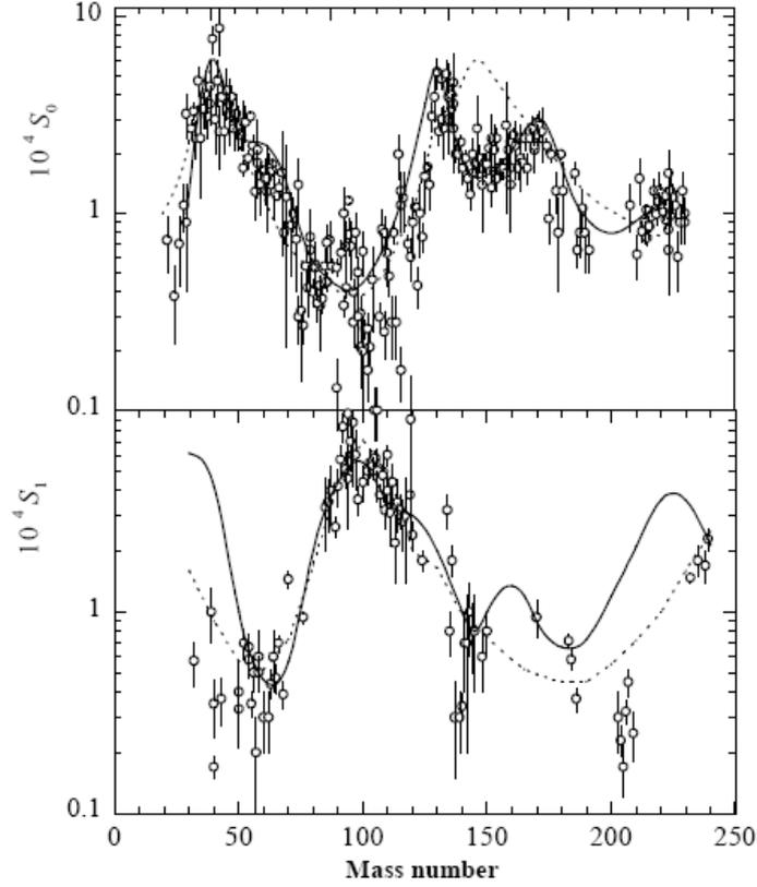
Fig. 6. Strength functions of  $s$ - and  $p$ -wave neutrons as a function of the mass number. Results of calculations are shown by dashed curves for the spherical optical model and solid ones for CCM.
