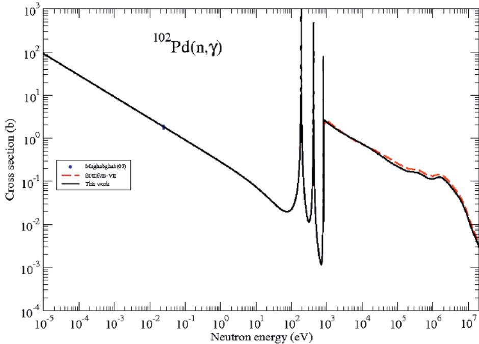
Fig. 10.  $^{102}\text{Pd}(n, \gamma)$  capture cross-section for the production of  $^{103}\text{Pd}$ .
