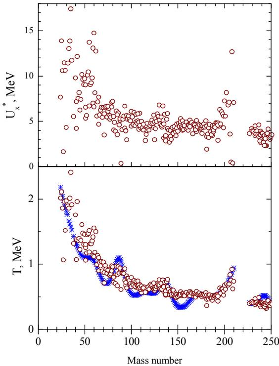
Fig. 3. Mass-number dependence on the nuclear temperature  $T$  and the effective excitation energy  $U_x$ , below of which the level density approximated with the constant temperature model. Blue crosses show the results of the independent analysis of the low-lying discrete levels.
