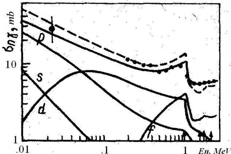
Fig. 1. Neutron capture cross sections for  $^{68}\text{Zn}$ , calculated taking into account the width-fluctuation corrections (solid curves) and without such corrections (dashed curve). The contributions of various partial waves are shown together with the corresponding experimental data for the total capture cross section (black symbols).
