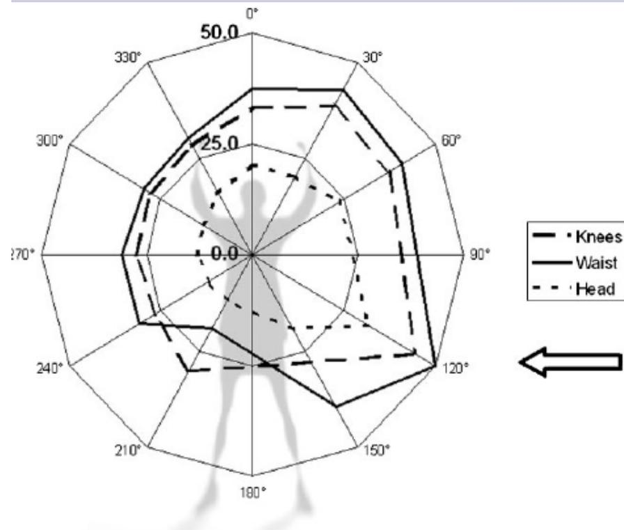
**Figure 8.** Distribution of scattered radiation from digital acquisition on the 10° right anterior oblique (RAO) projection at 68 kVp. The radial axis shows the dose in  $\mu\text{Gy min}^{-1}$ , whereas the ionization chamber position is indicated on the circumference. The figure shows the patient position from above, and the arrow shows the direction of the primary beam. Data for points not measured at 90°, 180° and 150° at 60 cm have been interpolated.
