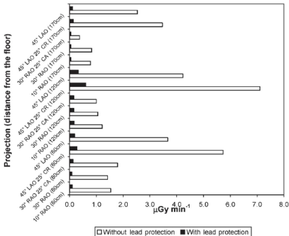
**Figure 4.** Measurements during fluoroscopy at the 210° position (cardiologist's position) with and without lead protection. RAO, right anterior oblique; LAO, left anterior oblique; CA, caudal; CR, cranial.
