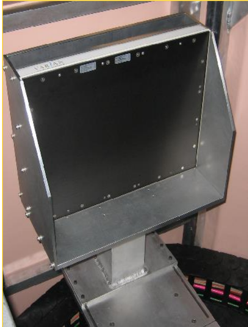
Varian 4030CB 194 \mu\text{m} pixels 2x2 388 \mu\text{m} 1024 x 768 x 30 FPS
