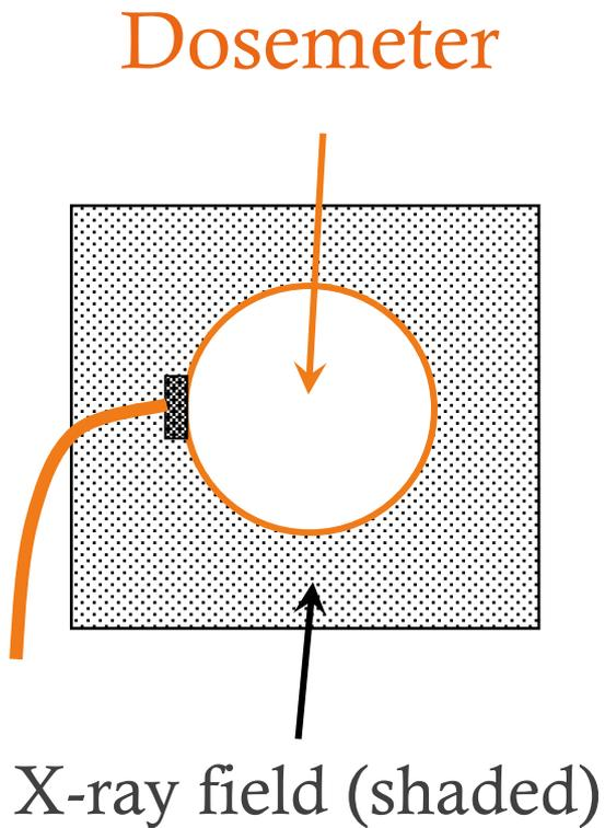
Air kerma measurements are made with the detector positioned entirely within the X-ray beam
