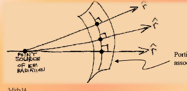
Portion of a spherical wavefront associated with a spherical wave
