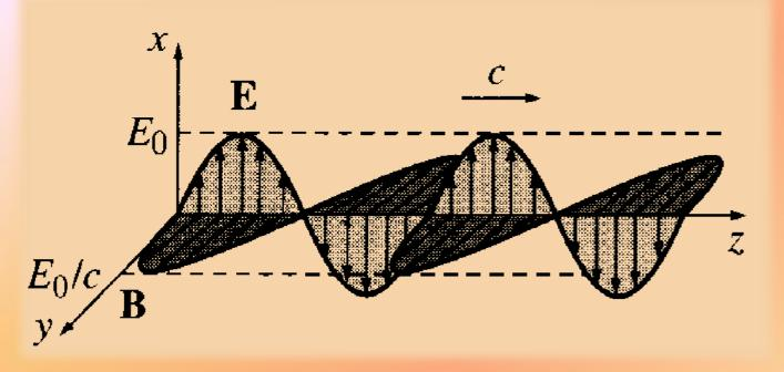
This is the paradigm for a monochromatic plane wave. The wave as a whole is said to be polarized in the x direction (by convention, we use the direction of E to specify the polarization of an electromagnetic wave).
