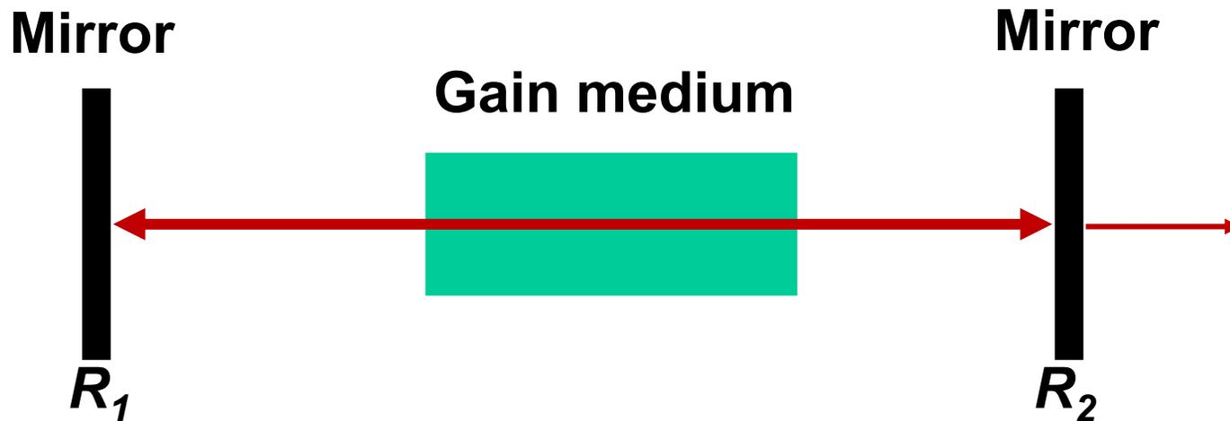
**Threshold**       $R_1 R_2 e^{2gL_g} = 1$
