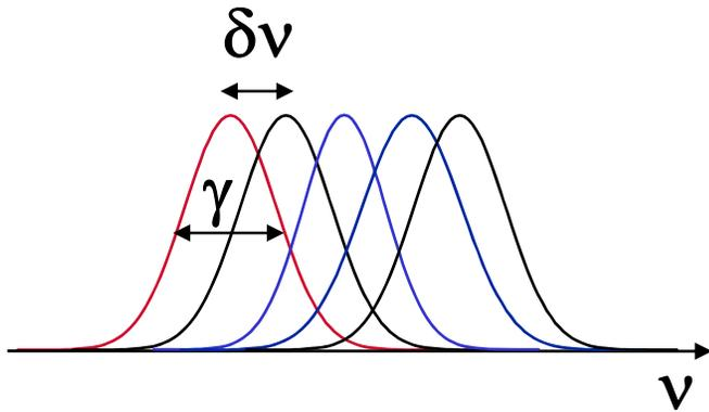
**Resonances are strongly overlapped spatially and spectrally.**
