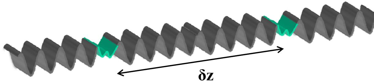
Temporal coherence length is determined by spectral bandwidth of laser emission
