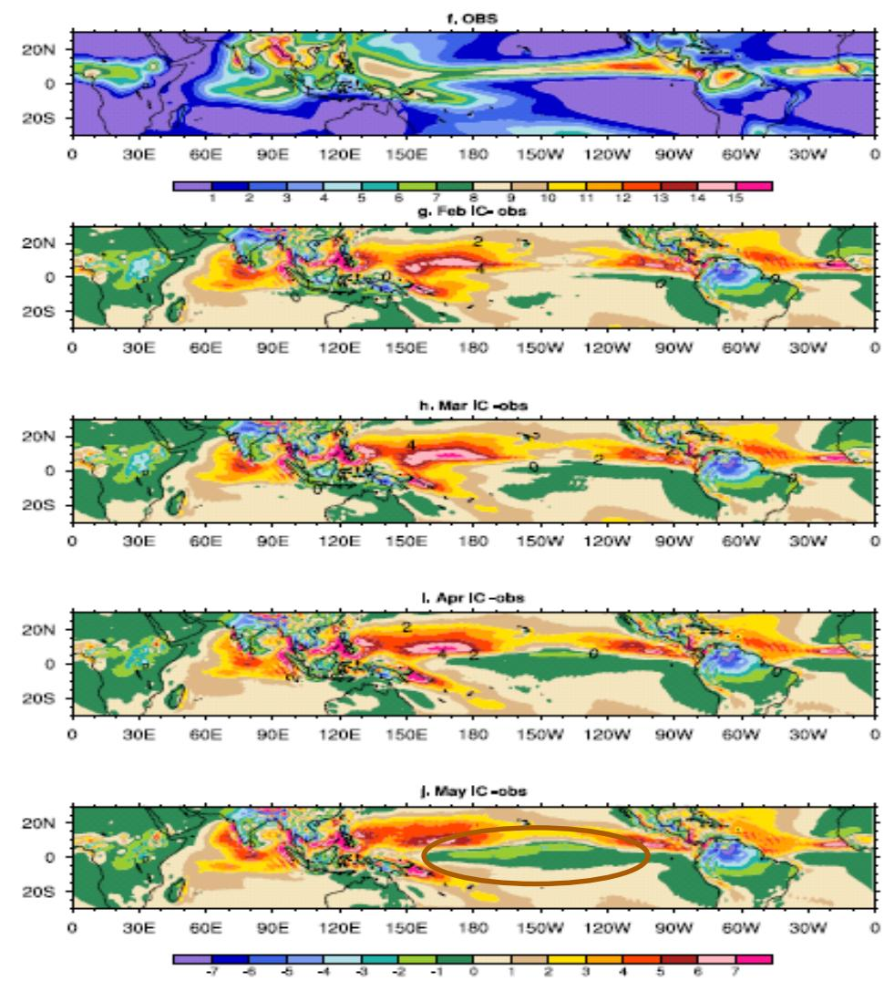
The JJAS climatology from Observed SST (a), and the climatological bias from observation for the CFS derived SST for Feb, Mar, Apr, May initial condition runs (b-e).(f-j) same as (a-b) but for precipitation
