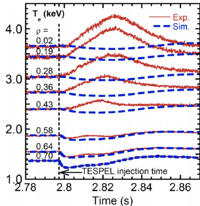
Propagation of perturbed  $T_e$  due to TESPEL in LHD
