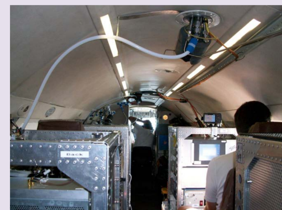
In left foreground, SPIRIT in the aircraft cabin, with the air sampling tube
