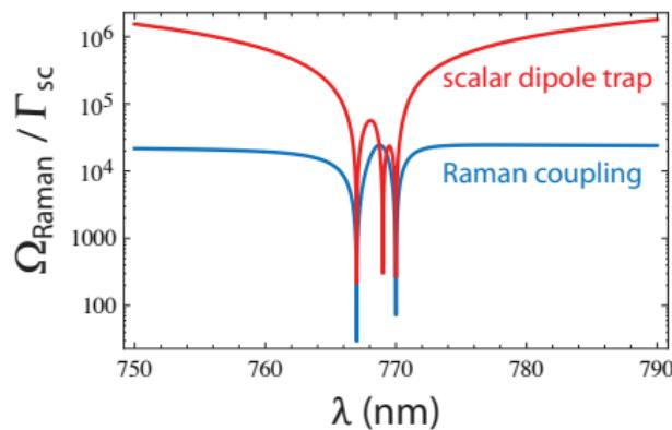
For an optimized detuning:  $\Omega_{\text{Raman}} = 1 E_r \leftrightarrow$  Heating rate of 700 nK/s.
