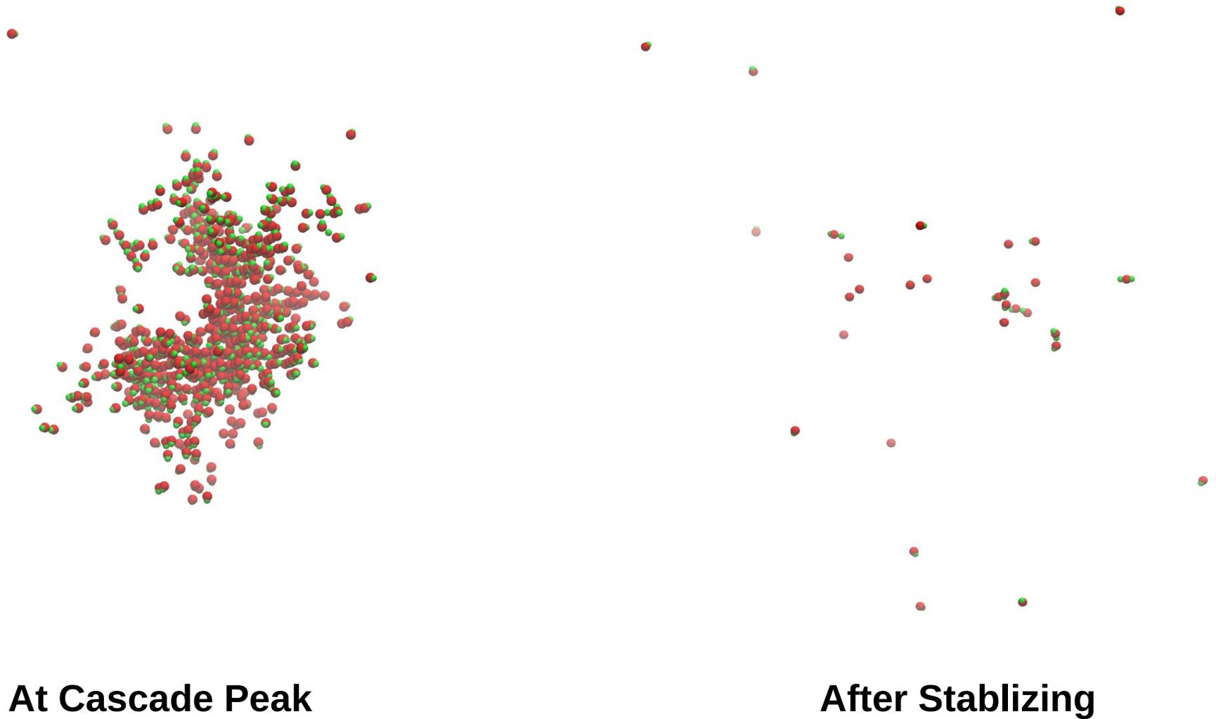
**Stoller - At peak interstitials are in close proximity which then recombine in an athermal process until steady state value is reached**
