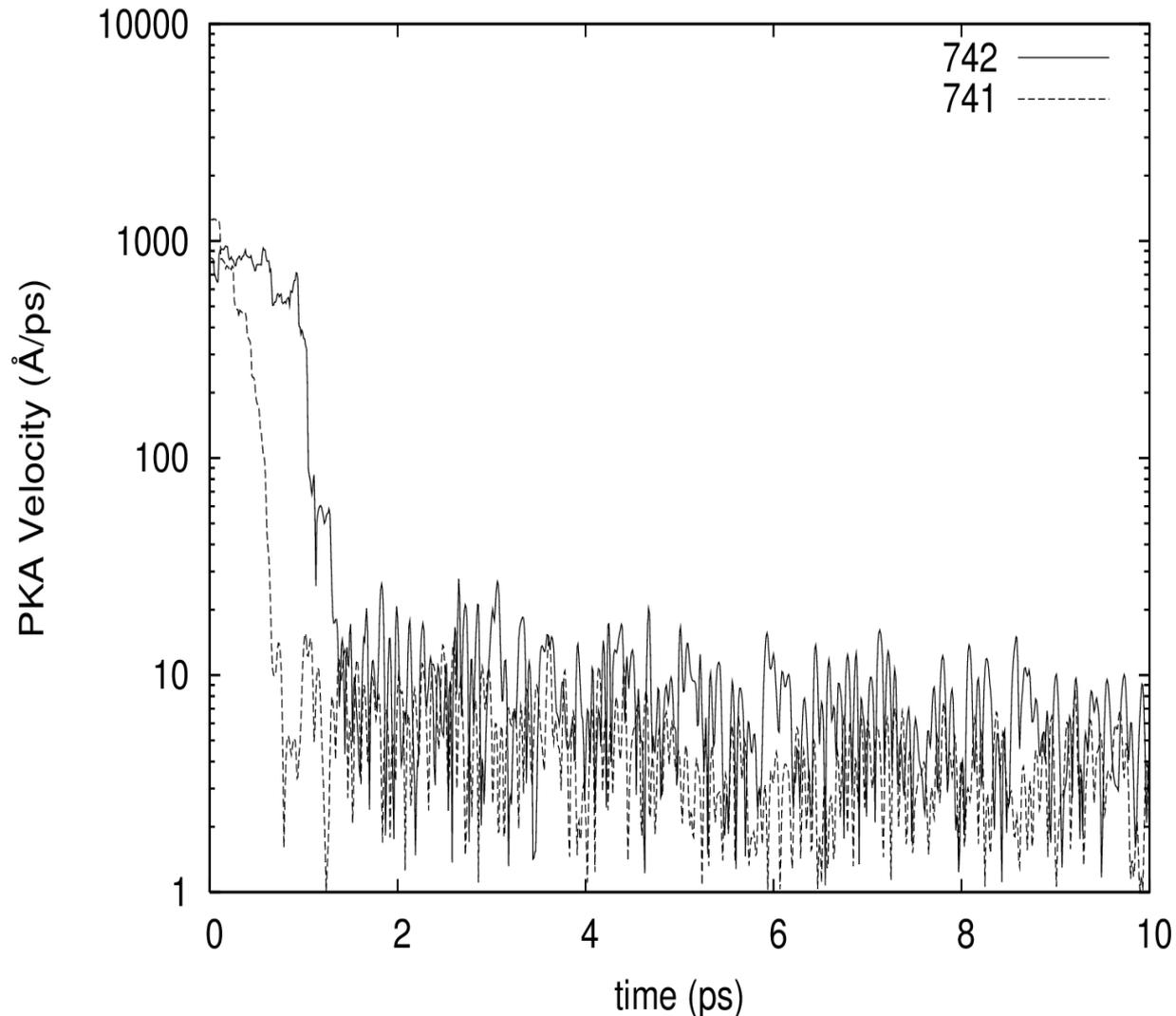
742<sup>nd</sup> PKA seems to have initially lost energy only in small angle collisions, thereby losing energy more slowly initially as compared to the 741<sup>st</sup> PKA
