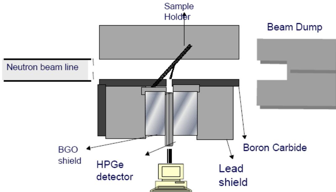
Fig.1 Schematic representation of the PGAA set up
