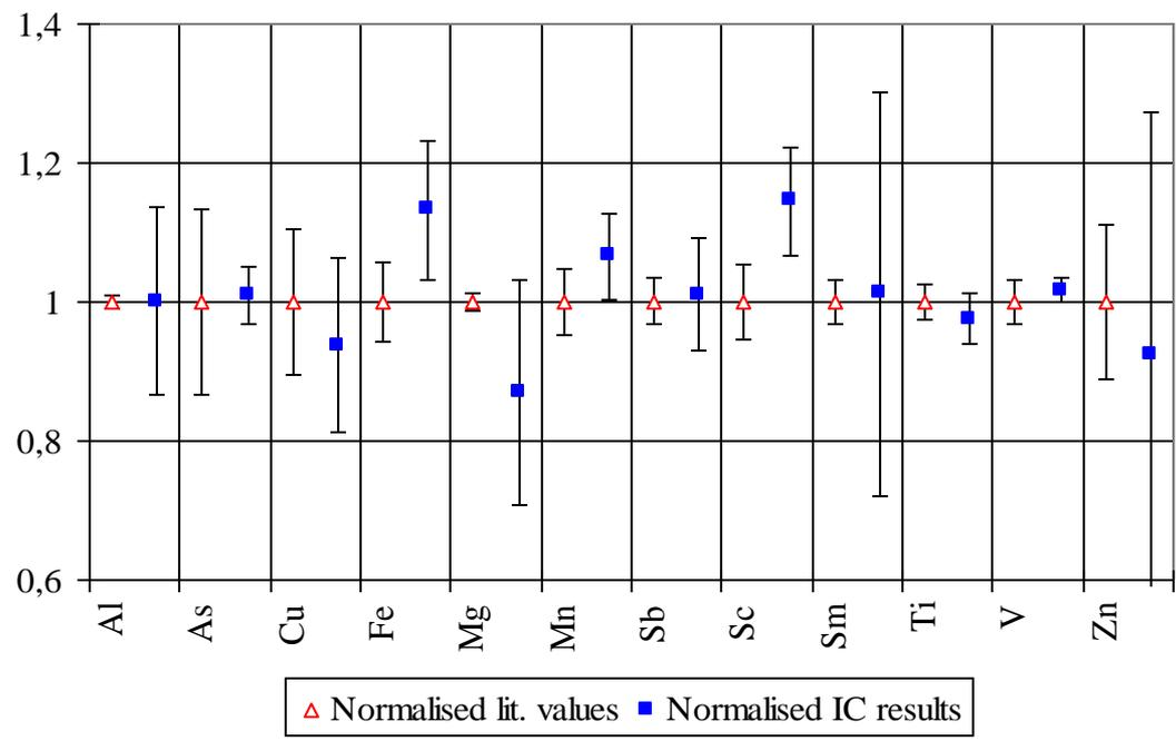
INAA means in lichen material. The error bars for the intercomparison results are standard deviations of the laboratory means.
