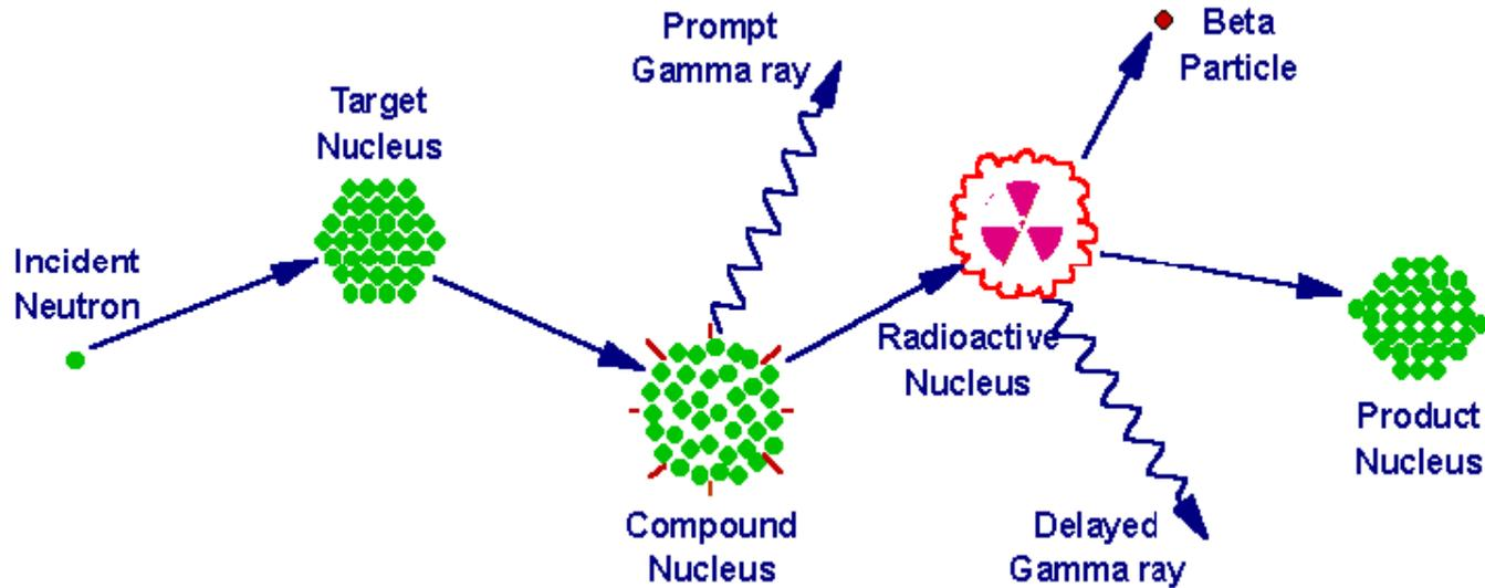
**NAA is a physical technique that is based on nuclear reactions. The sample becomes radioactive when neutrons react with the nuclei of the elements' atoms. Radioisotopes are formed and subsequently decay by emitting gamma rays that are unique in half-life and energy (identification). Gamma-ray intensity is proportional to the element content in the sample.**
