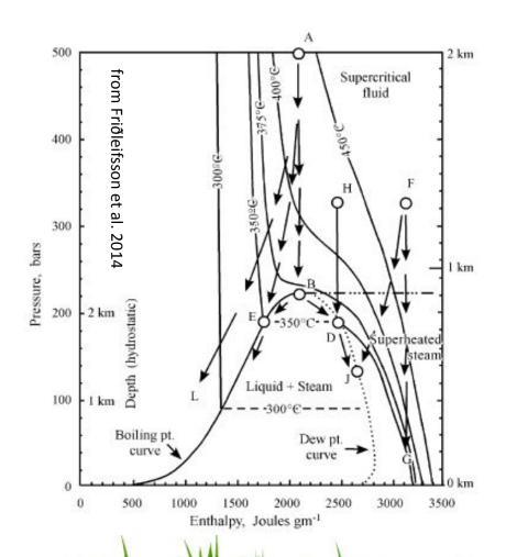
The enthalpy is one order of magnitude higher, per unit volume, than for a conventional hydrothermal fluid.
