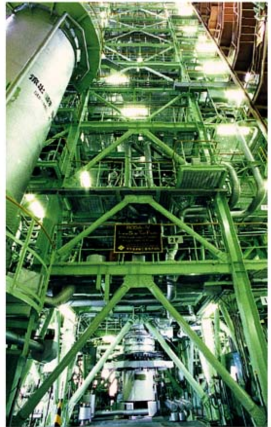
Large-scale Test Facility (LSTF): The world's biggest facility to simulate a PWR accident. More than 180 experiments have been conducted using the :LSTF and they confirm that Japanese nuclear power plants have adequate safety margins.
