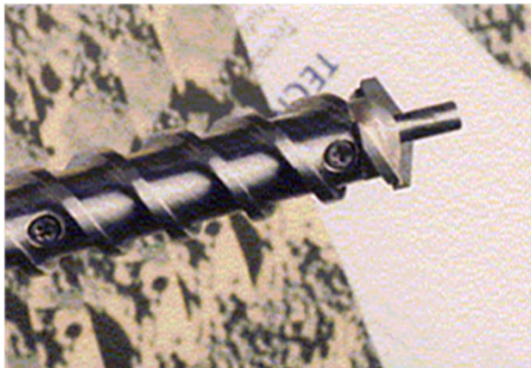
SD2 tip in sampling configuration
