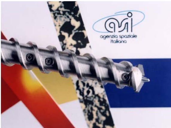
SD2 tip in drilling configuration
