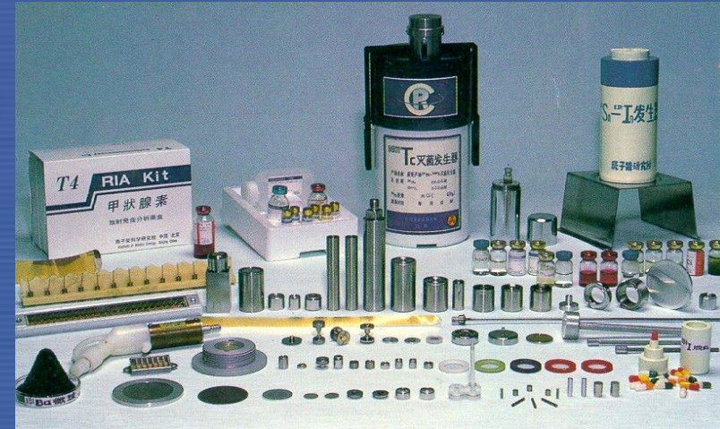
Typical forms of isotopic radioactive sources
