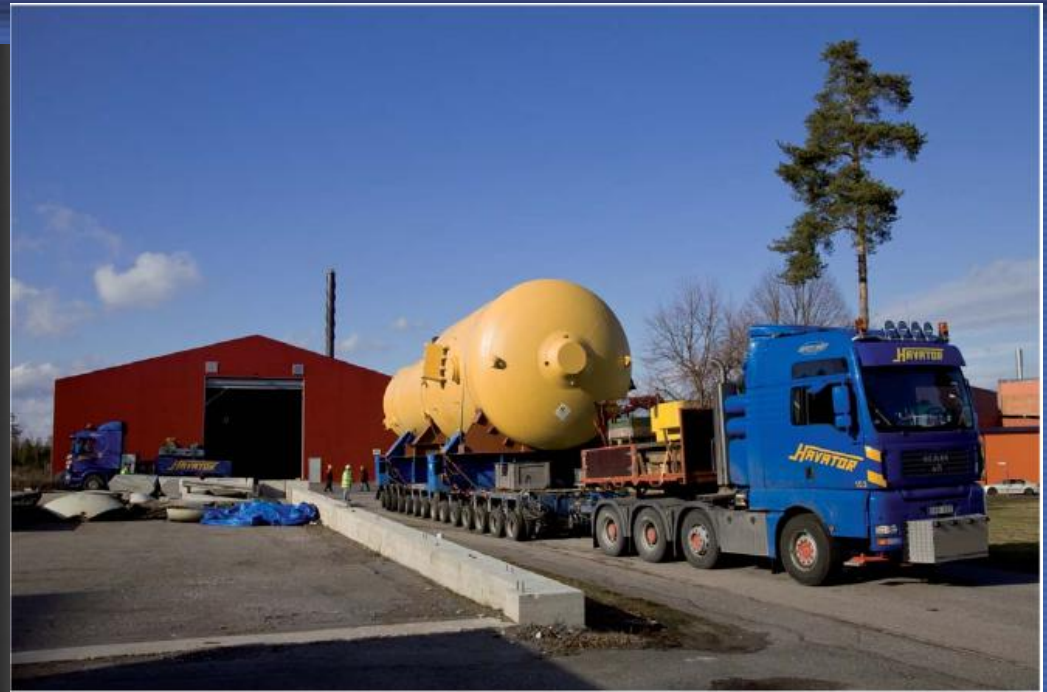
Redundant steam generator arriving for decontamination and metal processing Photo courtesy Studsvik
