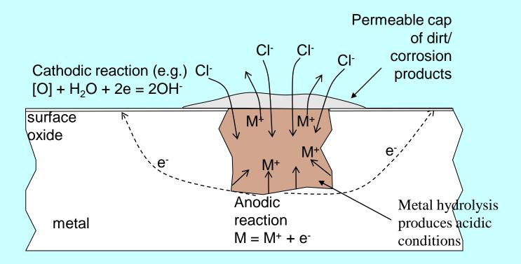
up to 10 microns/yr in seawater up to 1 mm/yr under accelerated conditions
